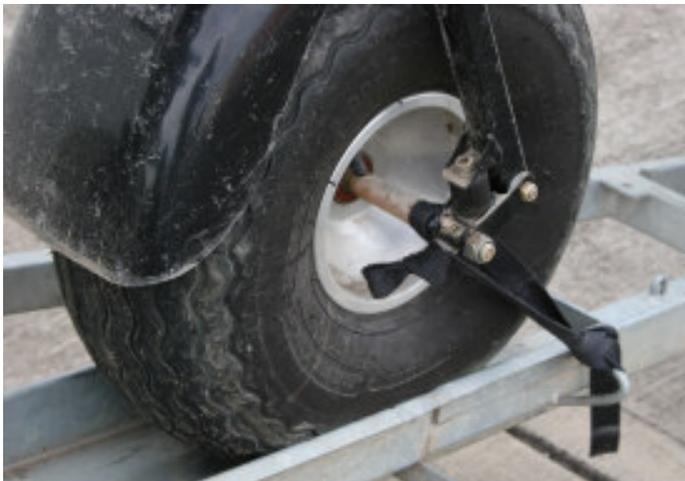
Figure 10 Front Wheel Tie Down
