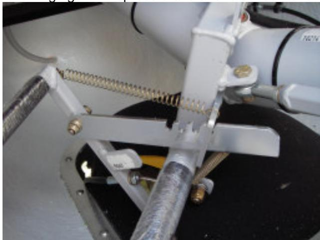
Figure 28 Brake Lock Lever.
