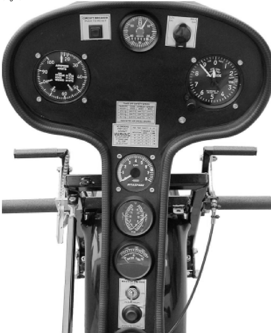
Top Row L to R:                    Circuit Breaker, Hour Meter, Power Outlet
