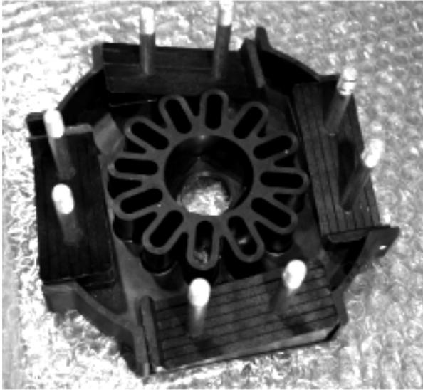
**Figure 49** Install blade retention bolts and pitch blocks
