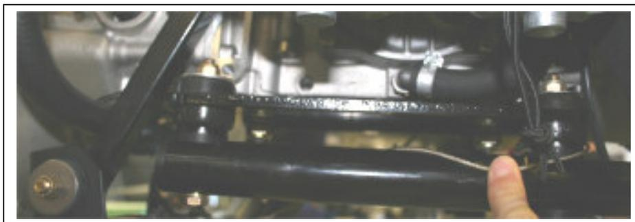
Figure 52 Engine Mount Rubbers (X 582 shown in photo)
