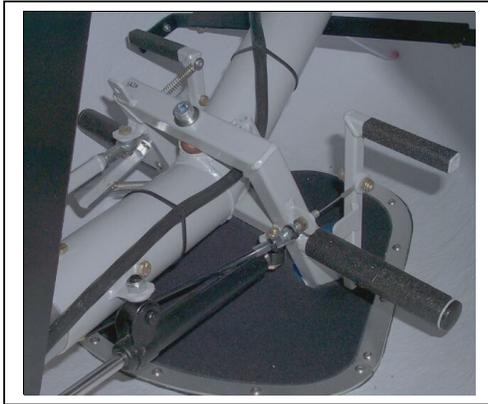
**Figure 33 Front Landing Gear Attachment**
