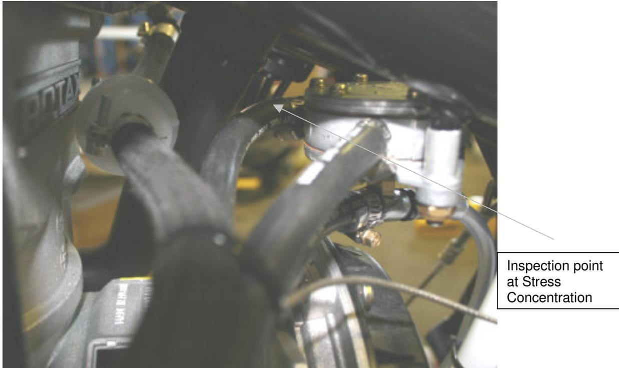
**Figure 23 Fuel Line Check Example**
