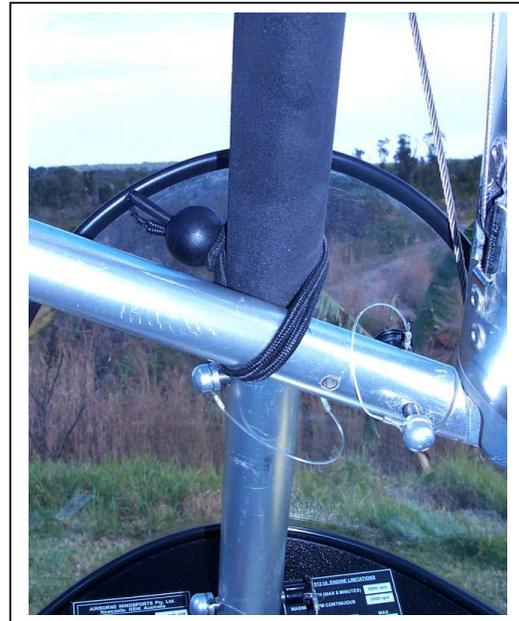
Figure 13 Securing of Base Bar With Rubber Shock Chord Fastener
