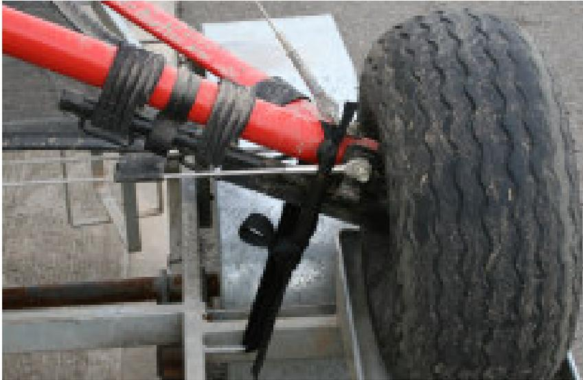
Figure 9 Rear Wheel Tie Down Location
