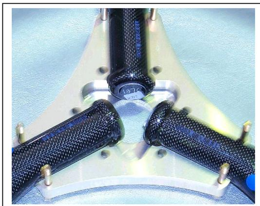
**Figure 39 Place Blades into Hub Block**
