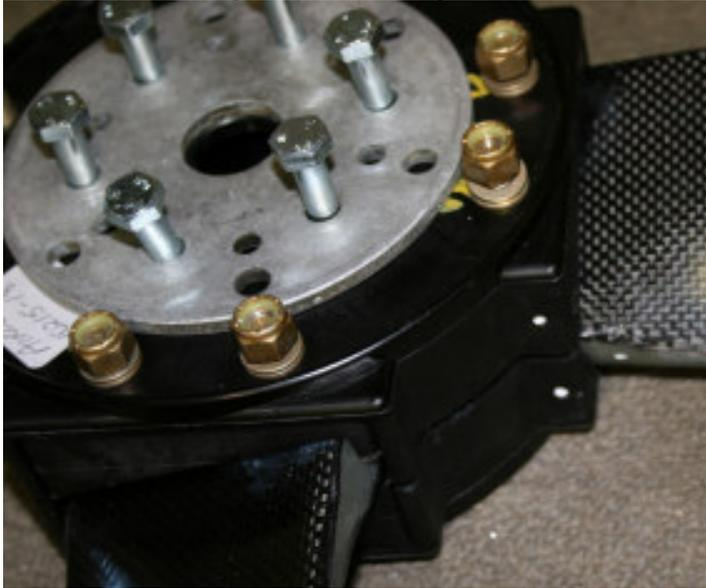
**Figure 51 Propeller hub assembly ready to torque the propeller blade retention bolt set**
